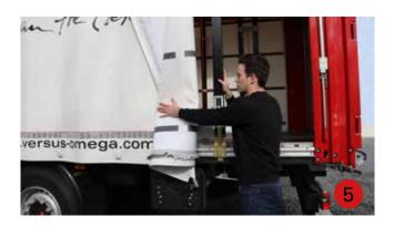
**6.** Pull the door stopper out, as demonstrated, to keep the system open.
